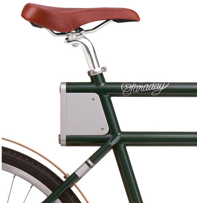
process of the electronic component box to incorporate flat surfaces. The VHB adhesive created a watertight seal for the electronic component box, and provided a long-term durable bond that would maintain its strength and secure the box for up to 35 years, regardless of outdoor conditions. After helping design the dimensions of the box, GMN die-cut four VHB gaskets in custom shapes to seal the box.
